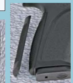
The field-stripped FNP-9 (l.) includes the pistol's one-piece polymer grip frame. Its generously flared magazine well aids rapid reloading of the double-column steel magazines.
