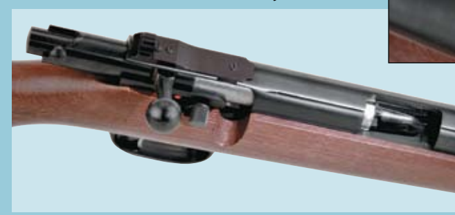
The Cub has a tubular steel receiver to which the barrel is pinned (below). The two-piece bolt has dual extractors, and the bolt handle is the locking lug, which engages a notch cut in the receiver when closed. The receiver-mounted ejector is fixed.
