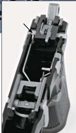
Linkage between the trigger and sear is by dual action bars. A projection on the right-hand bar (arrow) deactivates the firing pin safety as the trigger is pulled.
